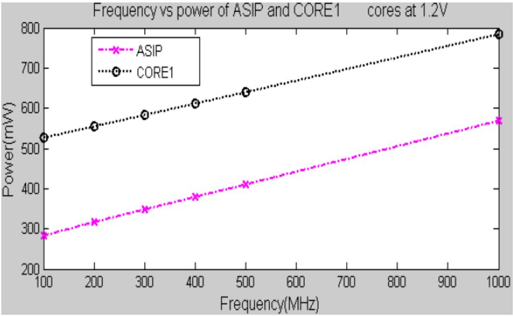
Fig. 6. Power consumption of ASIP and CORE1
