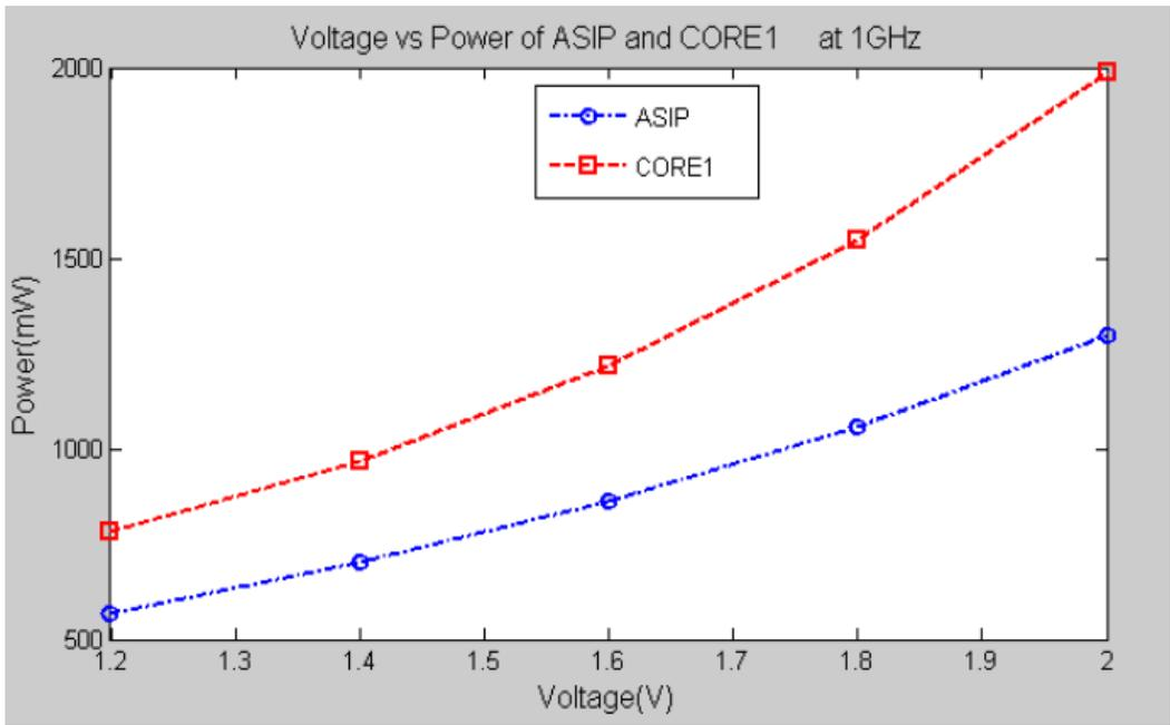
Fig. 5. Voltage vs power trend of ASIP and CORE1
