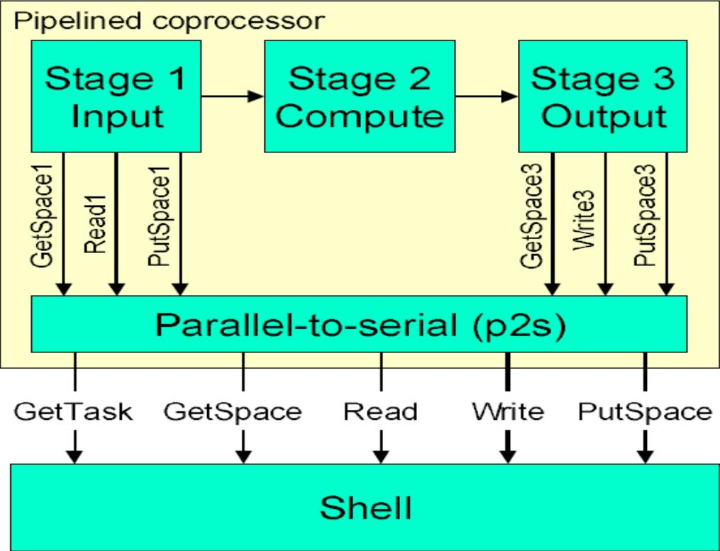
Fig.4. A model Pipelined Co-Processor
