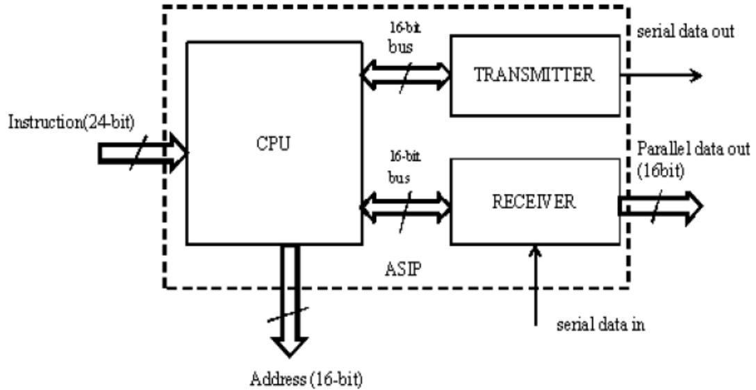
Fig.3. A Functional Block of ASIP
